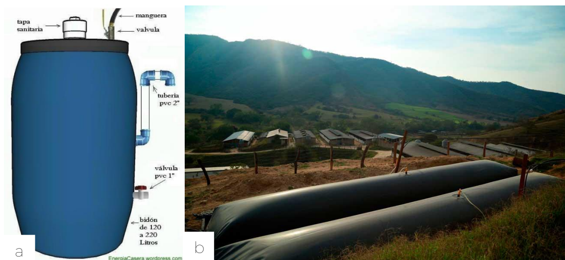
Figura 28: Biodigestores. (a) Biodigestor casero. ( https://s2.studylib.es/store/data/008945318_1-a4855b0c0fff4664599c1a57913d4d90.png ) (b) Biobolsa. ( https://www.teorema.com.mx/wp-content/uploads/impulsan-biobolsa.jpg )
